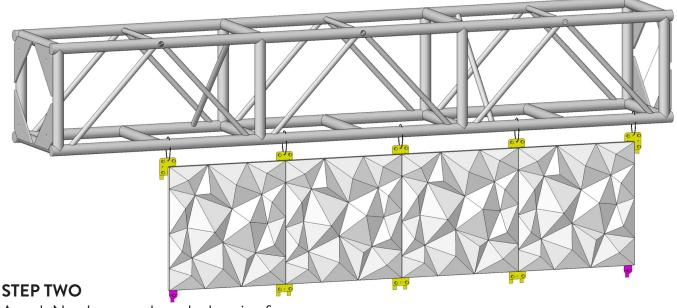
Attach No-show panels to the hanging fasteners.
