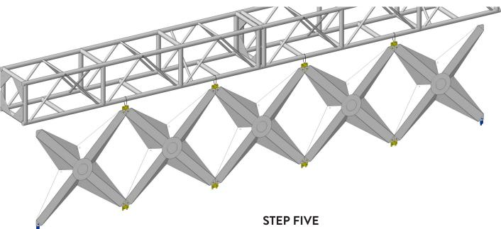
Connect Starburst together using F4 connectors
