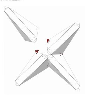
**STEP ONE** Assemble Starburst arms and connect using Flexi F2 connectors.
