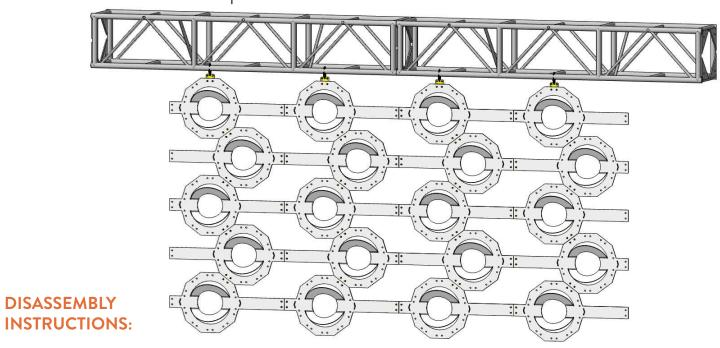
Backdrop MUST be disassembled from bottom up, in reverse order as the assembly process. Removal of top panels first may result in a collapsing wall.
