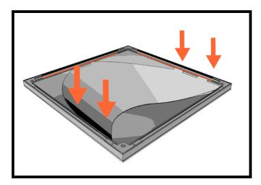
Bend Dune insert into fabric, lifting the frame to allow the insert to bend into the fabric. Place sides of Dune insert into frame channels or slots.
