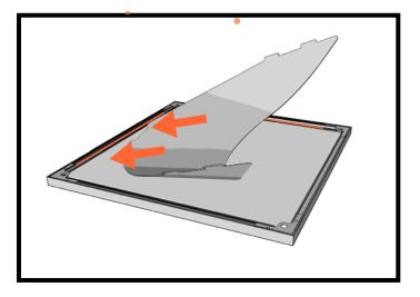
Place tabs into channel marked in orange.
