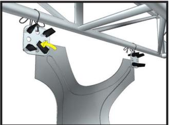
STEP FOUR Lock Connectors as you go Locked Position
